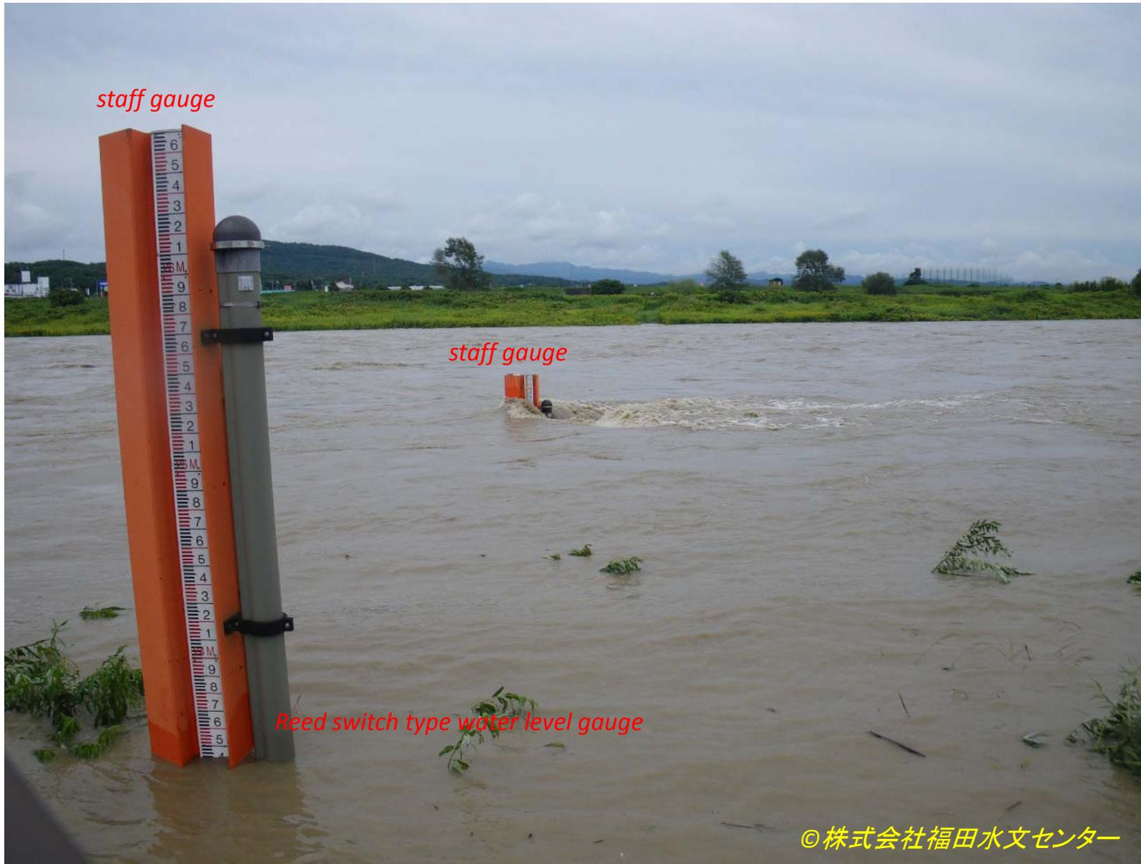
*Water level must be read on the staff gauge installed on the each section.*
