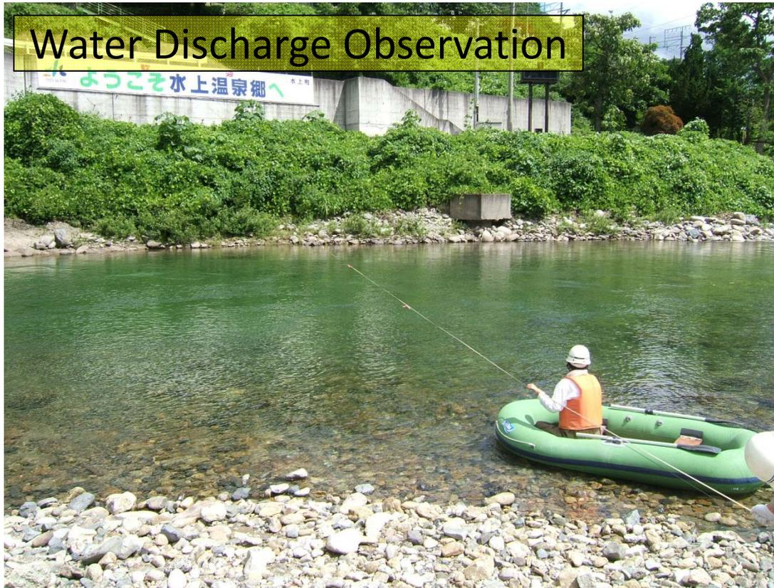
*Wire rope is stretched tight between both sides of river.*
