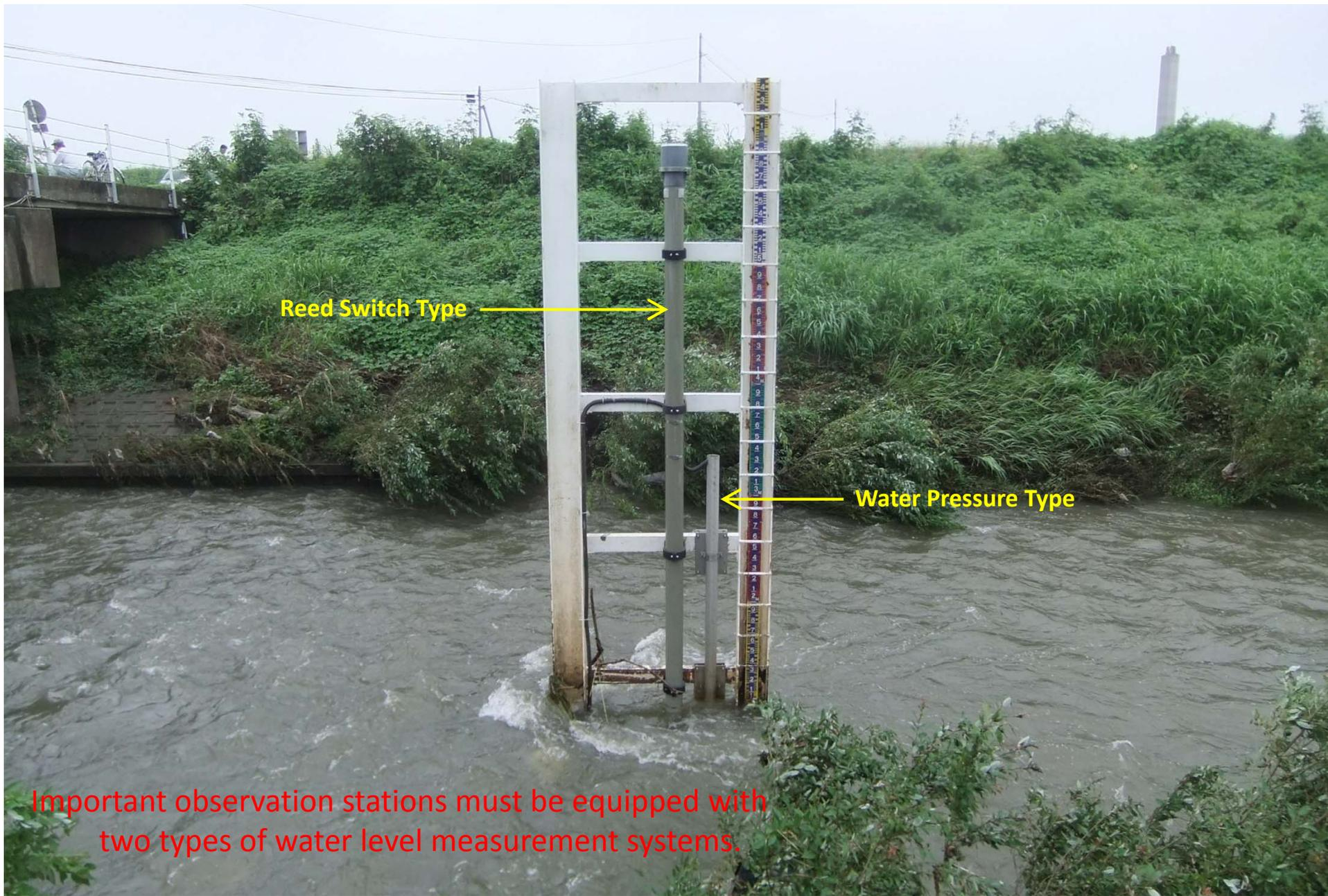
Important observation stations must be equipped with two types of water level measurement systems.
